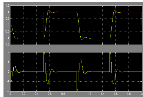
Figure 1.7 System response with CSMA/CD Network scheme Data rate 100000 bits/s frame size 10 bits with 0 loss probability
